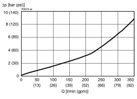
Dp = f (Q) Pressure drop - Flow rate characteristic Lowering B → A, valve fully opened
